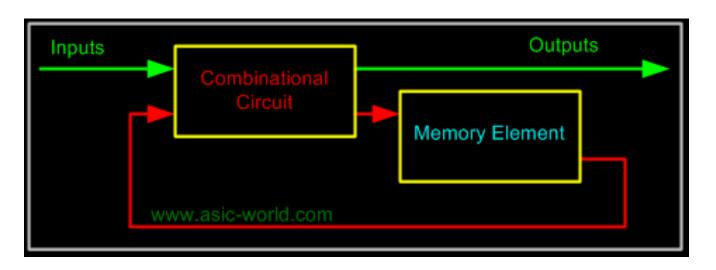
Combinational logic output depends on the inputs levels, whereas sequential logic output depends on stored levels and also the input levels.
