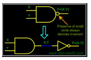
It has two or more inputs and only one output. The output of NAND gate is HIGH when any one of its input is LOW (i.e. even if one input is LOW, Output will be HIGH).
