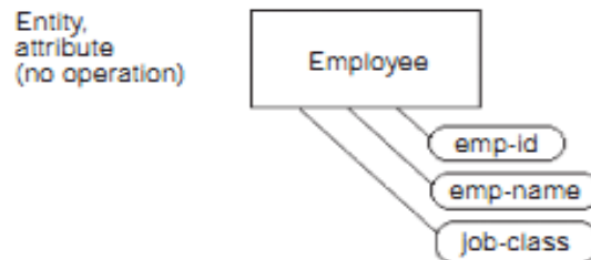
ER model constructs using the Chen notation
