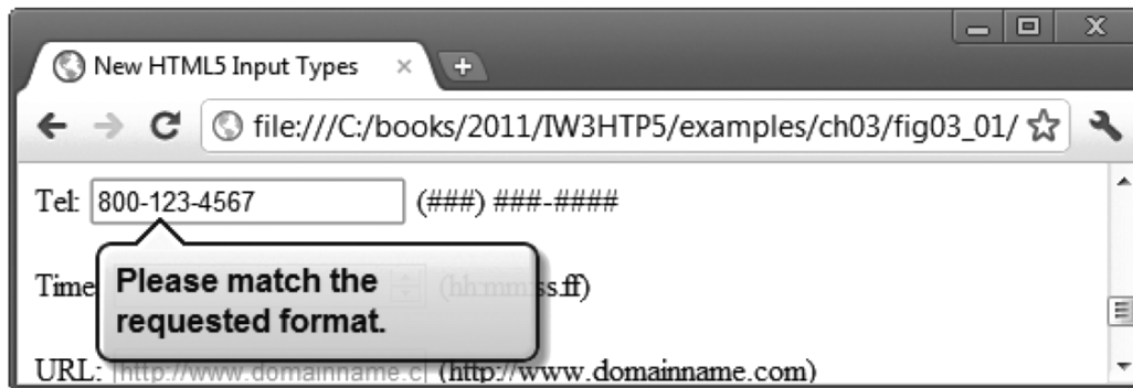
Fig. 3.14 | Validating a phone number using the pattern attribute in the tel input type.
