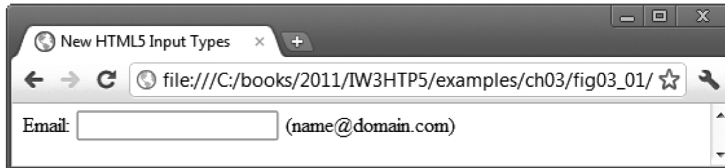
Fig. 3.8 | placeholder text disappears when the input element gets the focus.
