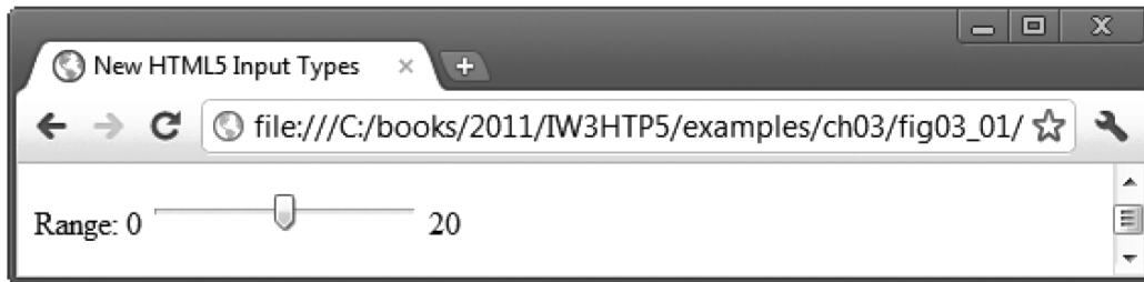
Fig. 3.12 | range slider with a value attribute of 10 as rendered in Chrome.
